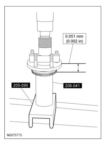
2. Using the Axle Bearing/Seal Plate and the Wheel Speed Sensor Ring Installer, press the rear anti-lock brake sensor on the rear axle shaft to specification.
