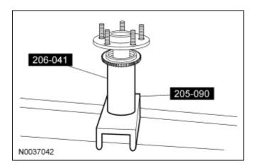
3. Install the rear axle shaft. For additional information, refer to Section 205-02A.
